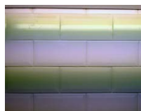
Photo with smartphone will show 'bands' if the light source has a low frequency
